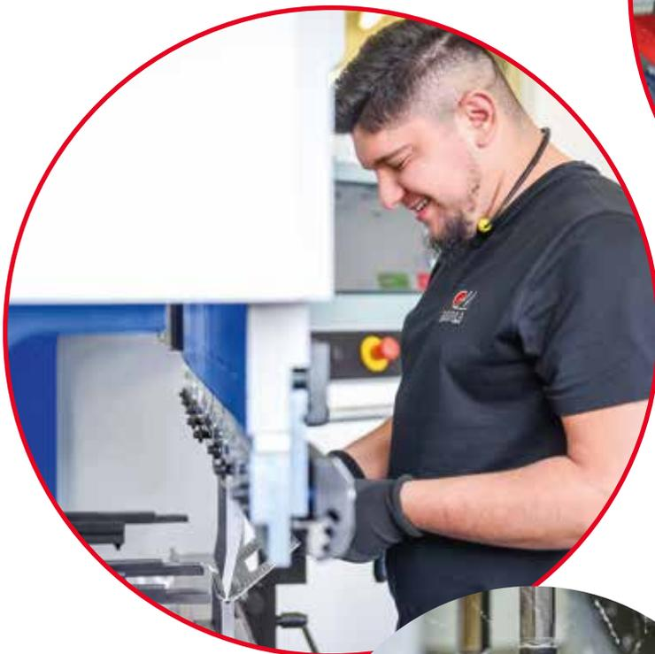
On request we manufacture individual enclosures using the stamping and bending process.
