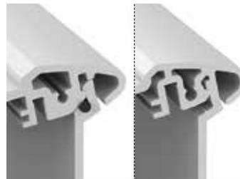
The factory-fitting of a round cord seal in combination with the AT...DI seal ensures that the ATPH variant (left) achieves protection class IP54. The ATPH-IP version (right) provides IP65 protection as standard.
