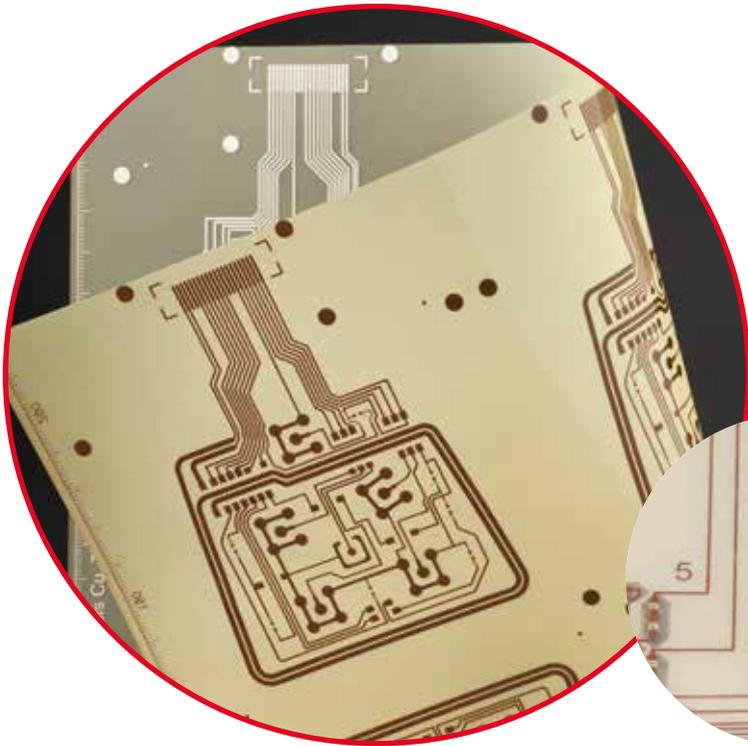
For demanding applications, we also create exclusive high-quality membrane keypads that incorporate the outstanding properties of surface-treated copper conductors.
