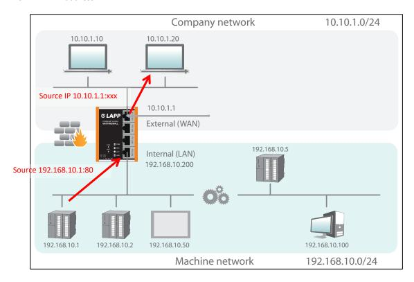
The option "NAPT: Active" thus enables communication of devices from the LAN with devices in the WAN. ETHERLINE® ACCESS NF04T thereby acts as a gateway to administer the implementation to the IP addresses of the WAN network and looks after the assignment of the response.
