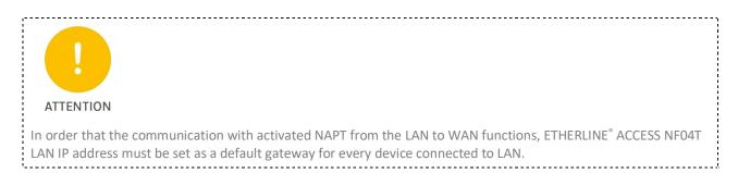
If the **NAPT** option is deactivated, the query packets from the LAN are forwarded from the LAN to the WAN with their original sender IP and sender port.
