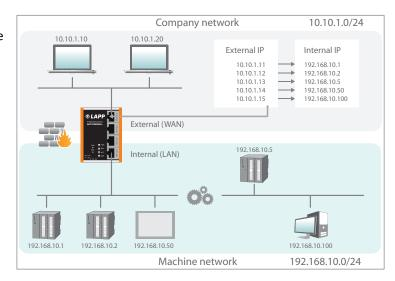
Broadcast traffic is generally filtered at the ETHERLINE® ACCESS NF04T, which means that the time behavior of the machine network is not impaired by the production network.
