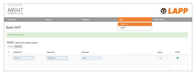
The "External IP" is the IP address under which the network participant of the machine becomes visible in the company/production network (WAN). The "Internal IP" is the IP address of the participant in the machine network (LAN). Any text can be entered as a comment.
