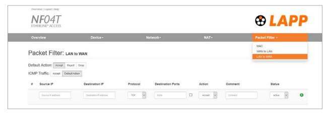
General rule can be changed by setting the "Default Action" to "Reject" or "Drop". In addition to general rule, filtering can be further customized using specific packet filter rules."
