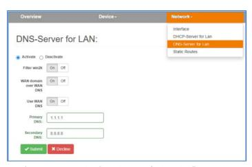
The DNS servers used by the ETHERLINE® ACCESS NF04T (Primary, Secondary) can be specified on the "DNS-Server for Lan" configuration page.
