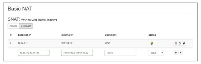
Using a subnet mask suffix to describe an entire IP range is also possible here: "10.10.2.1/24" defines a NAT rule for all IP addresses from 10.10.2.0 to 10.10.2.255.
