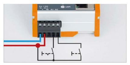
The inputs IN1 and IN2 do not yet have a function in the current firmware version but will be available in a later firmware version for the external switching of firewall rules.
