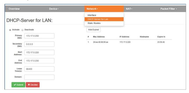
Primary/Secondary DNS: Specifies the IP address of a DNS server that is available to a DHCP client.
