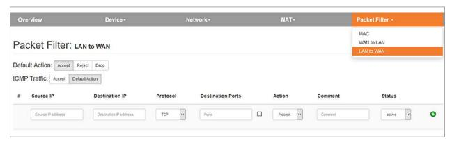
General rule can be changed by setting the "Default Action" to "Reject" or "Drop". In addition to general rule, filtering can be further customized using specific packet filter rules.
