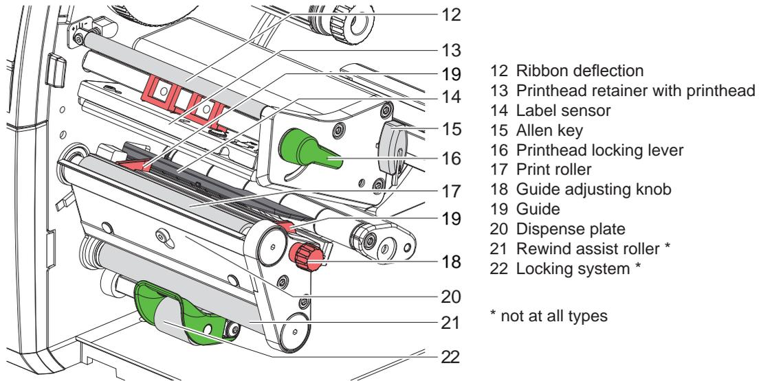
Figure 3 Print unit - devices with centered media guiding
