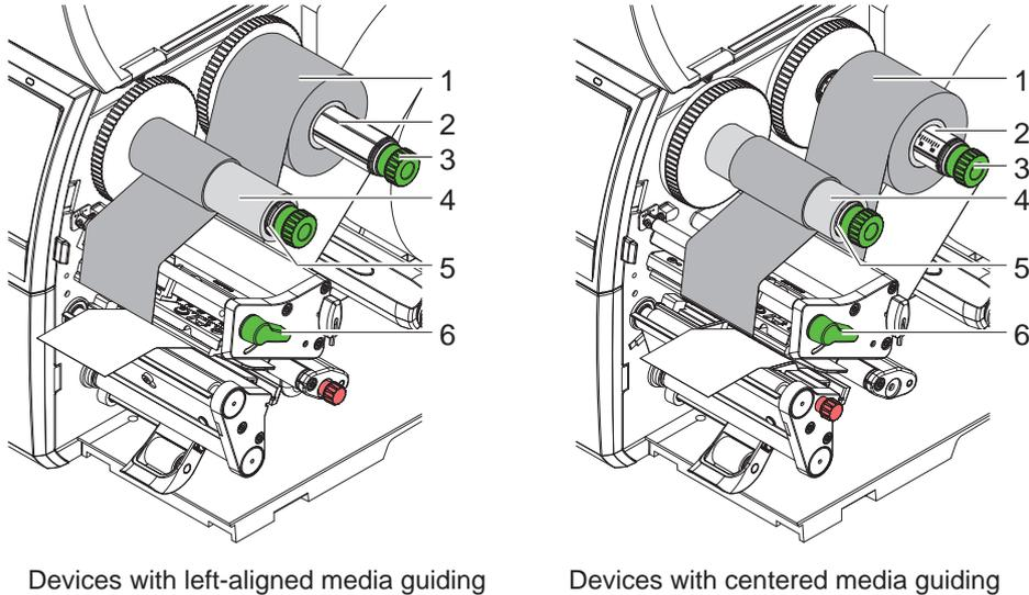
Figure 21 Loading transfer ribbon
