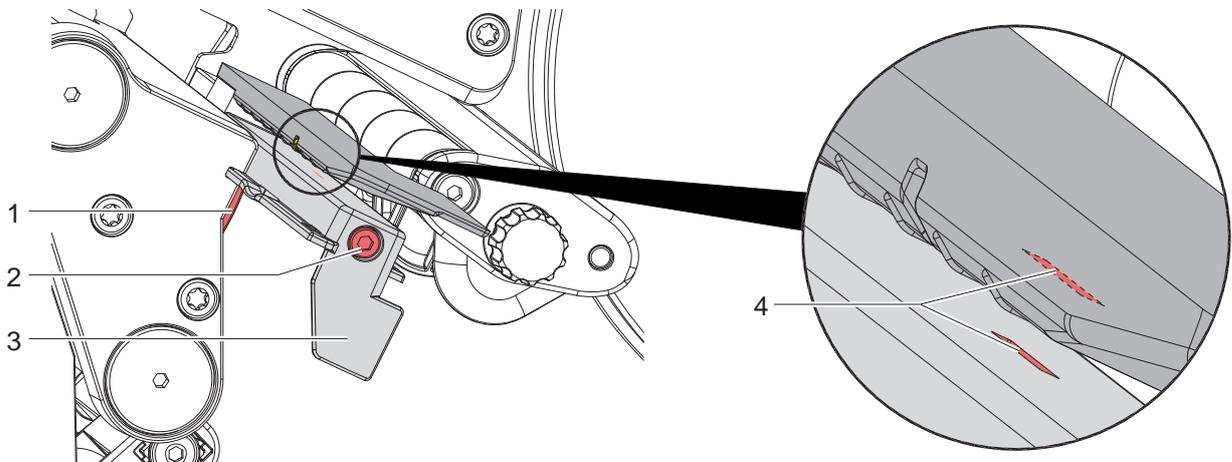
Figure 24 Cleaning the label sensor
