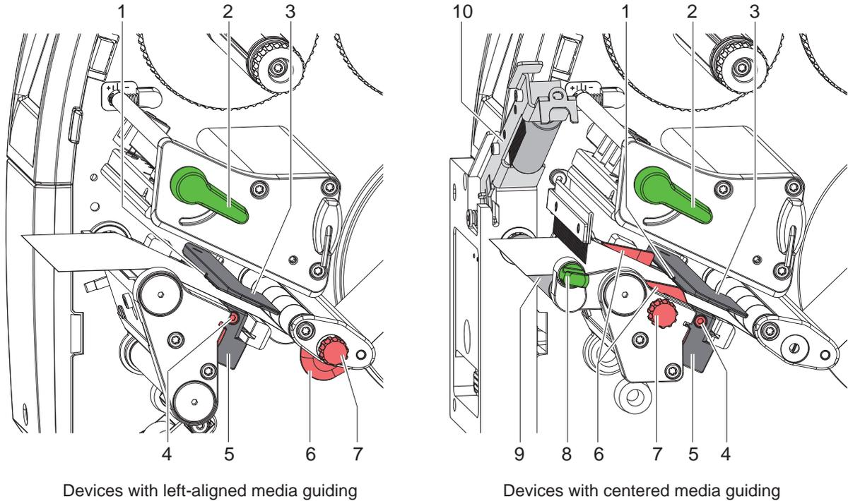
Figure 13 Inserting the media into the printhead
