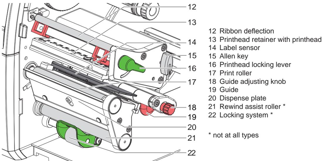
Figure 2 Print unit - devices with left-aligned media guiding
