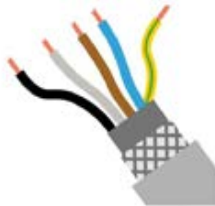
Figure 1: Simplified construction of a cable 1
